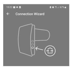
Activate the special setting mode on your device. To do this, hold down 'Ventilation' button on the device for 5 seconds until all LEDs start blinking, as shown in the figure above, and then click on 'Next'.
