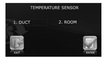
To change the temperature sensor, press the corresponding area on the LCD display and then press the ENTER
