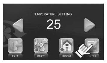
To set the desired temperature, use or buttons, then press the ENTER button to save the settings. To
