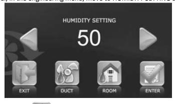
By pressing the DUCT or ROOM button you can chose the humidity sensor. DUCT humidity sensor is optional and is not supplied in the standard ventilation unit kit. ROOM humidity sensor is located on the LCD touch display.
