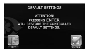
By pressing the ENTER button, the settings will be restored to default. By pressing the EXIT button, you will return to the engineering menu.
