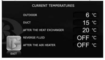
Current temperatures will be displayed, which are measured on the ventilation unit:
