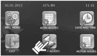
After pressing the TIMER ADJUST. button, the sub-menu for TIMER settings is displayed.
