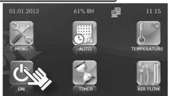
To activate or deactivate the ventilation unit, press the button ON to activate or OFF to deactivate the ventilation unit. When the ventilation unit is activated, the icon is highlighted in green, when the unit is deactivated the icon is highlighted in red. As long as the ventilation unit is deactivated, you will not be able to access menus and submenus or change any settings.
