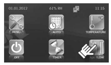
To set the air flow, press the button AIR FLOW, as shown in the picture above. With pressing the AIR FLOW button, you will enter the sub-menu for air flow settings, which enables four different settings:
