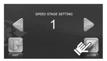
To select the desired ventilator speed, use or buttons, then press the ENTER button to save the settings.
