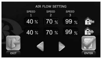
Choose the ventilator speed, which you want to adjust; press on the corresponding LCD display area, the chosen
