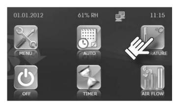
After entering the temperature setting sub-menu, the temperature sensor can be chosen, according to which the ventilation unit will function.
