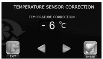
button change the value for the temperature correction and then press the ENTER
