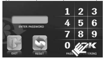
After entering the password press the OK button. If you have entered the wrong password, press the RESET
