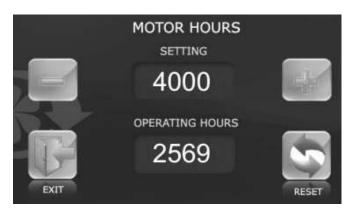
Then with or buttons change the interval duration for filter maintenance. The window OPERATING HOURS displays the current operation time of the ventilation unit since the last filter maintenance. After the filter maintenance
