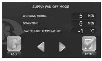
By pressing on the corresponding area on the LCD display, you can choose WORKING HOURS, DOWNTIME and SWITCH-
