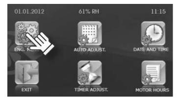
Access to engineering menu is only possible with a password. The password is factory set to 1111.
