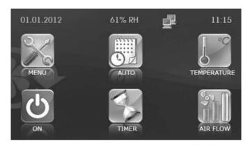
In the upper part of the main menu, from left to right, current date, current air humidity and time are displayed. From the main menu, all functions and sub-menus can be accessed. Also a status icon for internet connection is displayed in the upper part of the main menu:
